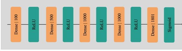
**Fig. 2:** Proposed neural network structure. The number in each dense layer indicates the number of neurons being used.
